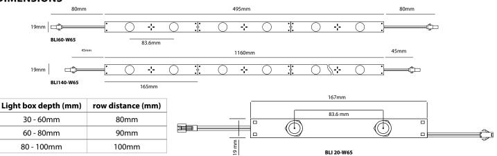
Results may vary depending on face material properties. The data above was obtained using 3mm thick opaque acrylic with a 54% light transmittance. Lucoled advises to paint the inside of the box/letters in a matt white colour for achieving an optimal result. Always test before production.
