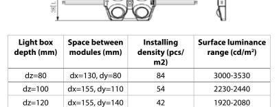
Results may vary depending on face material properties. The data above was obtained using 3mm thick opaque acrylic with a 54% light transmittance. Lucoled advises to paint the inside of the box/ letters in a matt white colour for achieving an optimal result. Always test before production.
